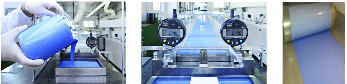
Casting of a LTCC slurry according to the Heraeus Deutschland GmbH & Co. KG formula.
